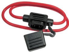
Micro 2 Fuse Holder With Dust Cap & 12" Wire #0959 - 16 GA 10 AMP #0960 - 12 GA 30 AMP
