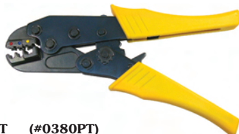
#0380T (#0380PT) Ratchet Crimping Tool Crimps 22-18, 16-14 & 12-10 Ga Terminals 3 Separate Crimping Nests
