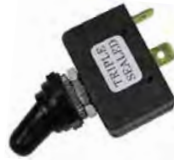
#5513C (#5513PT) On-Off Toggle w/Boot Nut 2 Position - 2 Terminal 3/4" Handle Length 2 1/4" Male Tabs Moisture Proof Metal Body - Dipped 12 Volt 20 Amp
