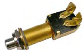
#5527C (#5527PT) Marine Push-Button Momentary On SPST Starter & Horn Switch Chrome Plated Brass 2 Screw Terminals 5/8" Mount Hole 6 Volt 25 Amp 12 Volt 15 Amp
