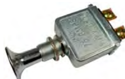
#5522C (#5522PT) On-Off Push-Pull SPST Heavy Duty Chrome Plated Metal Knob 2 Copper Terminals with 2 Brass Screws 1/2" Mount Hole 6-28 Volt 75 Amp
