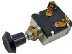
#5521C (#5521PT) On-Off Push-Pull SPST 2 Screw Terminals 1/2" Mount Hole 6 Volt 25 Amp 12 Volt 15 Amp
