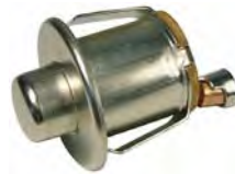
#5508C (#5508PT) Universal Starter Switch Grounded Snaps Into 15/16" Hole 6 Volt 15 Amp 12 Volt 10 Amp 24 Volt 6 Amp
