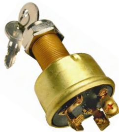
#5529C (#5529PT) Brass Heavy Duty Ignition Starter Switch 3 Position - 3 Screw Terminals 13/16" Mount Hole 6 Volt 25 Amp 12 Volt 15 Amp
