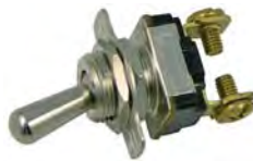
#5576C (#5576PT) On-Off Toggle SPST 1/2" Metal Bat Handle With Indicator Plate 1/2" Mount Hole 120 VAC 6 Amp 240 VAC 3 Amp
