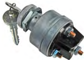
#5503C (#5503PT) Ignition Switch - 2 keys Accessory-Off-Ignition-Start 30 Amp 3/4" Mount Hole Plated Steel w/4 Terminal Studs
