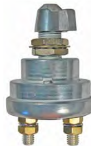
#5574C (#5574PT) Master Battery Disconnect 2 Stud Terminal 3/4" Mount Hole For Battery Circuit Only On - Off SPST 6-36 Volt 190 Amp DC Continual 1000 Amp DC Momentary
