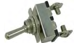
#5578C (#5578PT) Momentary On-Off Toggle SPST 5/8" Metal Bat Handle With Indicator Plate 1/2" Mount Hole 12 Volt 20 Amp
