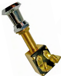
#5528C (#5528PT) Push-Pull Brass Switch SPST w/2 Position Tabs Chrome Plated Knob 2 Screw Terminals 3/8" Mount Hole 6 Volt 25 Amp 12 Volt 15 Amp
