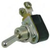
#5510C (#5510PT) On-Off Toggle SPST 3/4" Metal Bat Handle 1/2" Mount Hole 12 Volt 15 Amp 125 VAC 10 Amp
