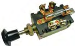
#5514C (#5514PT) Push-Pull Headlamp Switch with 15 Amp Fuse 3 Position Off-On-On 5 Screw Terminals 3/8" Mount Hole 12 Volt 15 Amp
