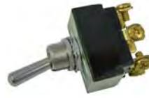
#5558C (#5558PT) Moment On-Off-Moment On DPDT Toggle 3/4" Handle Length 6 Screw Terminals 12 Volt 25 Amp 125 VAC 20 Amp
