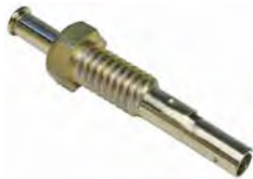
#5506C (#5506PT) Door Jamb Switch Self Grounding 3/8" Travel Length 2" Overall Length 12 Volt 1 Amp
