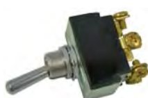
#5549C (#5549PT) On-Off-On Toggle DPDT 3/4" Handle Length 6 Screw Terminals 12 Volt 25 Amp 125 VAC 20 Amp
