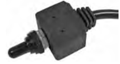
#5589C (#5589PT) Momentary On-Off- Momentary On Toggle SPDT - 3 Position Waterproof w/Boot 3 6" 16 Ga Wire - Jacketed 1/2" Mount Hole 12 Volt 25 Amp
