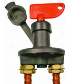
#5575C (#5575PT) Isolator Switch (See Page 20) Theft & Fire Protection 2 Position On-Off 12 Volt 7/8" Mount Hole Includes Removable Key Moisture Proof Cap 350 Amp DC Continual 500 Amp DC Momentary
