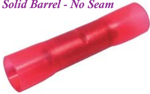
Strip Wire - Insert Into Barrel - Crimp Apply Heat Until Adhesive Flows & Tubing Shrinks
